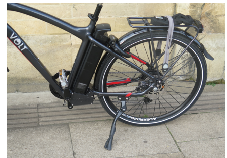
The battery is fitted just behind the seat tube, while the hub motor can be seen in the centre of the back wheel.
