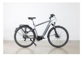
The Infinity's intuitive Shimano Steps drive system reads and matches riders' effort, providing power that blends into every rider's style. Combining the power of this motor with the intelligence of the fully automatic electric Shimano Alfine 8-speed gears, Volt says the Infinity is its most sophisticated bike yet.
