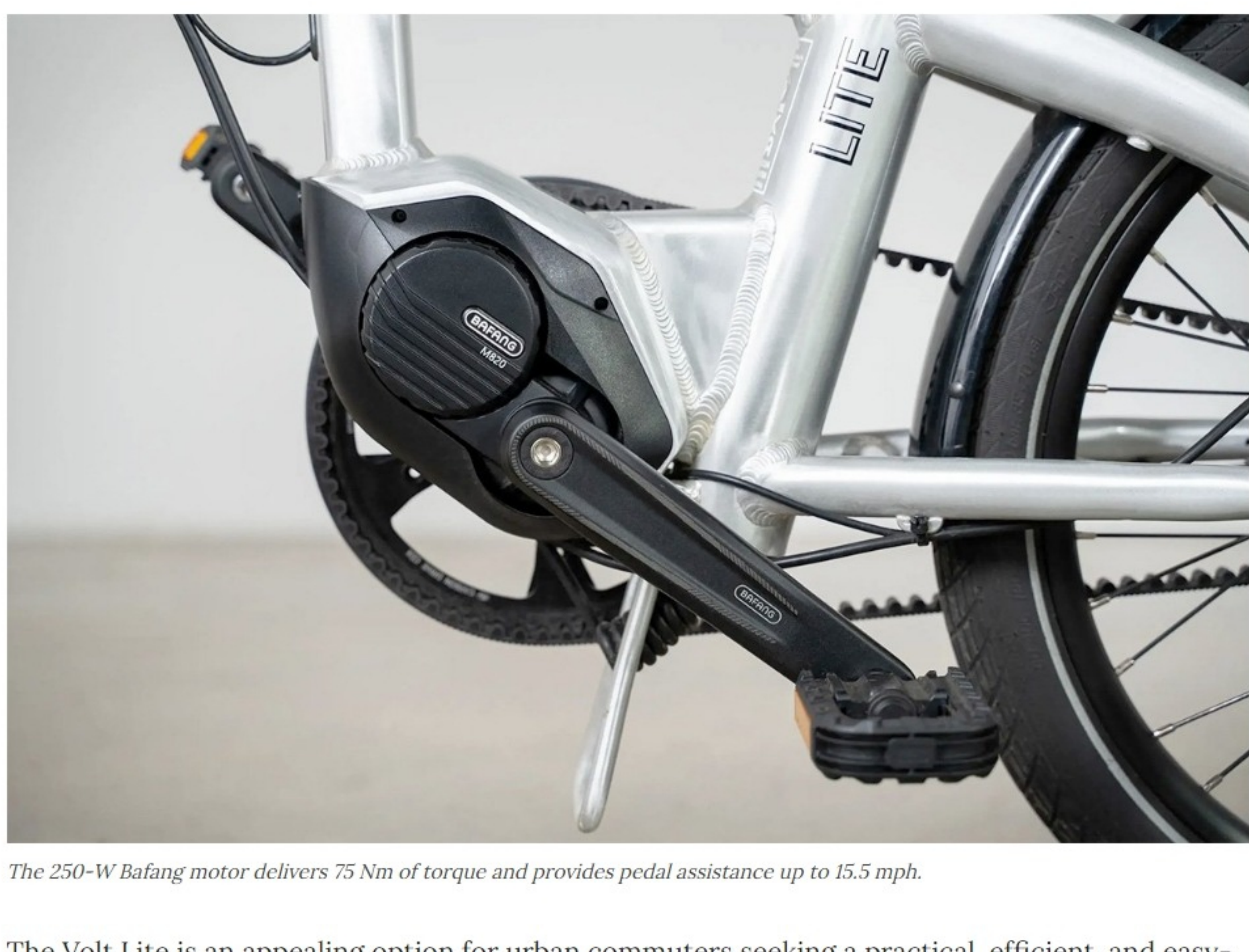
The 250-W Bafang motor delivers 75 Nm of torque and provides pedal assistance up to 15.5 mph.
