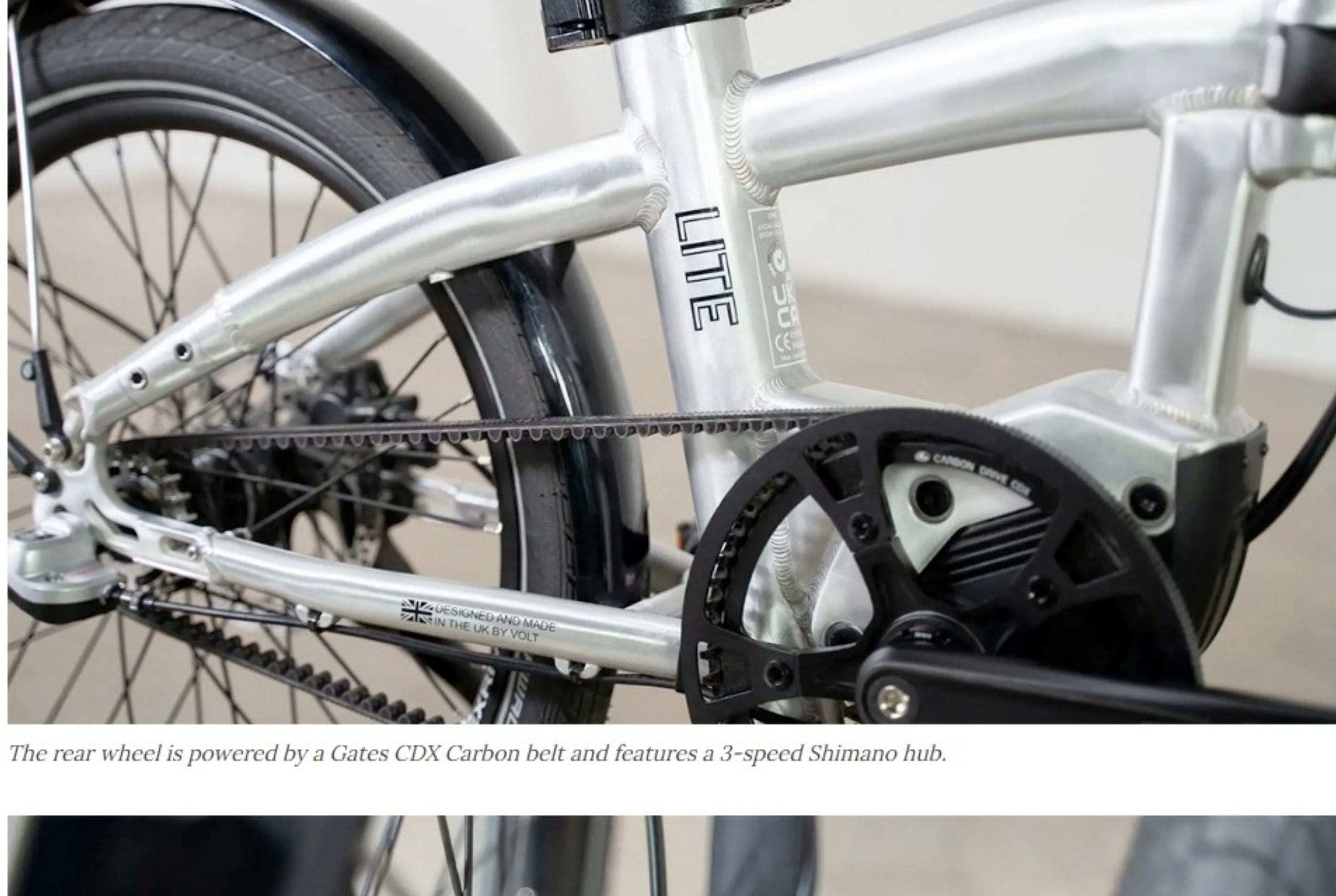
The rear wheel is powered by a Gates CDX Carbon belt and features a 3-speed Shimano hub.
