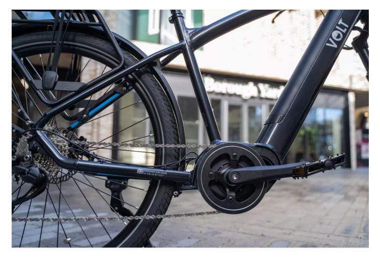
Priced at <u>£2,699 the Connect's</u> stand-out feature is its crank-mounted Bafang motor. Crank drive is a really nice thing to have on an e-bike, because it delivers the power very smoothly, which gives makes for a much more natural riding feel. The propulsion is carefully measured, depending on your riding style, and based on the amount of torque you're putting into the pedals, the gradient you're riding on and the speed you're travelling.
