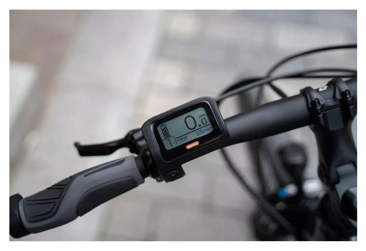
And those settings are controlled by a compact handlebar-mounted display, with a few discreet buttons that will take you through the power settings, at the same time as giving you statistical readouts and displaying battery life.
