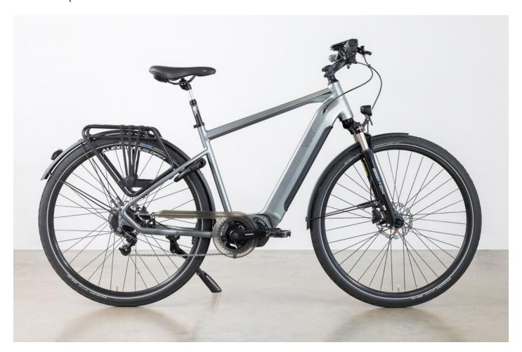
The 504Wh battery is built into the frame and offers 90-plus miles of electric assist. It can be charged on a domestic connection in around three-four hours.
