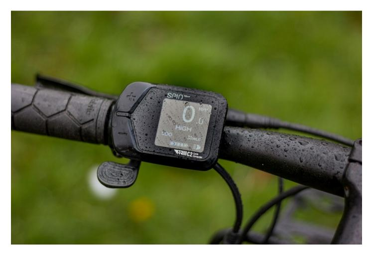
The London is pretty much ready to ride. It comes with Spanninga front and rear lights which are activated on the control unit on the handlebars. This is also where you control your assist levels. Mudguards are pre-installed – something I was very grateful for given the weather, and there's a bell on the handlebars, too.
