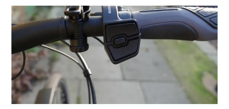
With gear shifting provided by Shimano, the Infinity also has an all-electronic gear system that lets you swap up and down using buttons on its handlebars.
