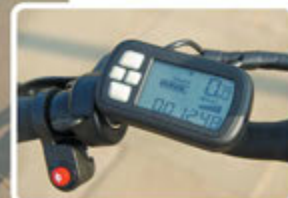
BELOW: The LCD display gives a clear view of parameters including speed, distance, battery status and assist level.
